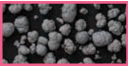
Average particle size: 54 \mu\text{m}
