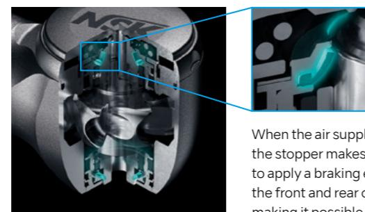
When the air supply is stopped, the rubber of the stopper makes contact with the rotating shaft to apply a braking effect. With stoppers attached to the front and rear of the head, contact is increased, making it possible to abruptly stop the rotation.
