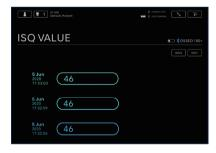
When the ISQ value is measured with Osseo 100+ under this condition, the ISQ value displayed on the control unit is also displayed on the screen of the terminal. Touch "SAVE" to save the ISQ VALUE data to the terminal storage and the PDF is automatically displayed.
