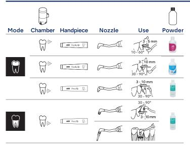
1) Hold the powder handpiece. 2) Select the powder mode (Prophy 🗑 / Perio 🗑 ). 3Set the power level. 4 Adjust the irrigation level. 5 Depress the ON / OFF button.
