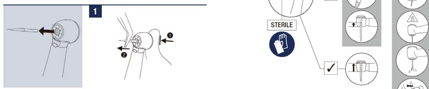
**WARNING** If blood or debris is stuck, wipe in and around the bur insertion hole with a cloth moistened with disinfectant solution until all residues are thoroughly removed. Residual blood or debris may enter the handpiece while changing burs, which could lead to higher risk of cross-contamination.
