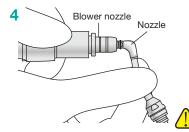
Use the blower nozzle in the same way to clear the lines in the Perio-Mate nozzle. Blow from the far end of the nozzle.
