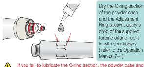
Dry the O-ring section of the powder case and the Adjustment Ring section, apply a drop of the supplied turbine oil and rub it in with your fingers ( refer to the Operation Manual 7-4).
