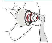
Replace the O-ring(s) at the handpiece joint section of the powder case, apply a drop of the supplied turbine oil and rub it in with your fingers.
